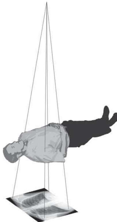
Figure I.2 The creation of a two-dimensional projection through the body. In this case, x-rays are transmitted through a patient creating a radiograph.
