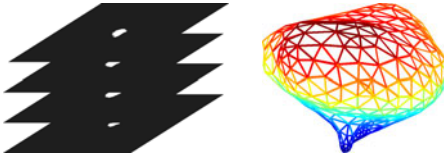
Fig. 2. Generating a 3D mesh for the lung nodule surface from a stack of successive segmented 2D LDCT slices
